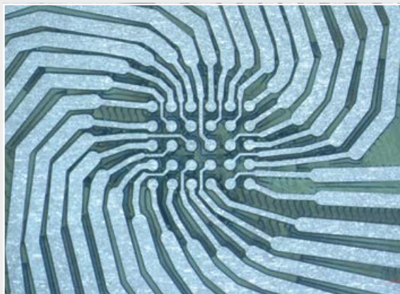
Fanout on Dupont AC 354500R for gadgets
