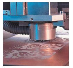
From left to right: AMS's AM1010H Airmagic<sup>™</sup> Handsfree Wireless Headset for mobile devices , AMS Design Verification/Accelerated Life Test Lab with compliance verification apparatus and test solution, and close-up view of an LPKF C30 ProtoMat<sup>™</sup> plotter milling a precision circuit board.
