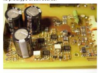
Fig. 1: Milled and Populated Prototype Board
