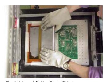
Fig. 6: Manual Solder Paste Printing
