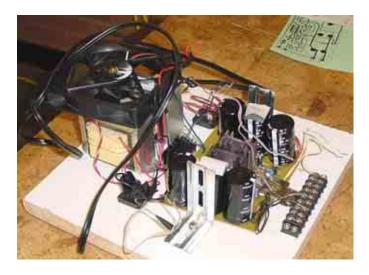
Assembled amplifier circuit
