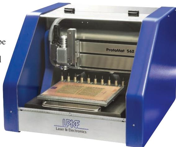
**2. The ProtoMat S62's 10-bit auto changer permits continuous, automatic operation with a host of tools.**
