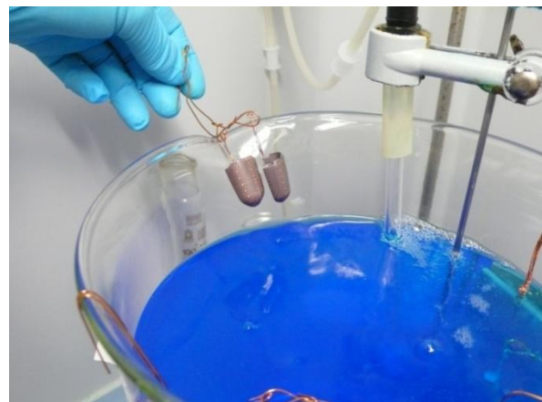
The laser-structured components can be chemically metallized in an industrial-scale process or – as shown here – in cascading beakers. A base layer of copper and a finish layer of nickel/gold are standard.
