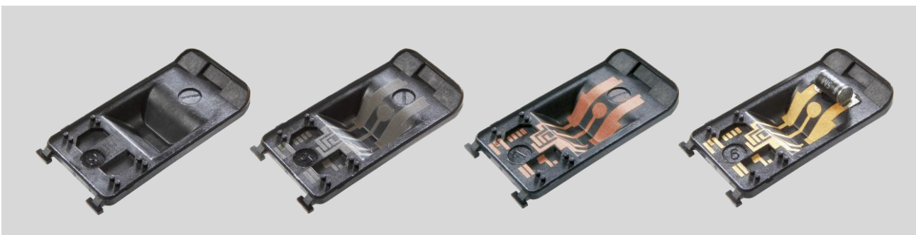
LDS (left to right): The injection-molded part (1) is structured by laser (2) and then metallized (3). Components and contacts can be mounted on the metallized surface (4).
