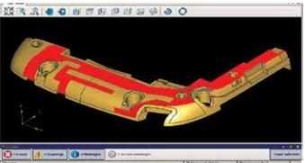
The LDS process 'writes' circuits onto parts with a laser beam striking the molded part's plastic surface.
