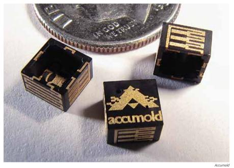
This sample part is approximately 1/4" square and is molded with a platable PC/ABS-blended resin. The parts were laser-treated on all six sides and are plated with a final gold finish.
