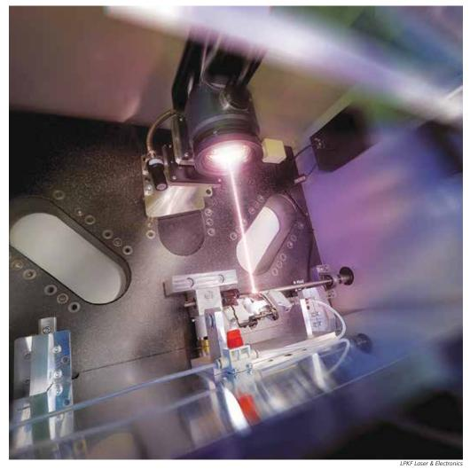
The laser direct structuring process makes it possible to produce circuit layouts on 3D structures.
