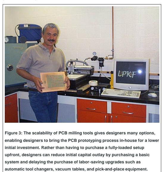
Alternatively, they can reduce their capital outlay by purchasing a basic system and delaying the purchase of labor-saving upgrades such as automatic tool changers, vacuum tables, and pickand-place equipment (see Table 1). This enables designers to bring the PCB prototyping process in-house for a lower initial investment.
