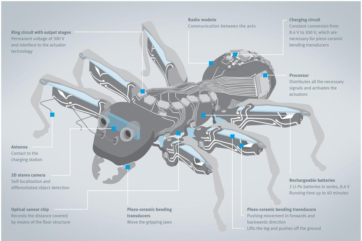
The BionicANTs also come very close to their natural role model in terms of design and constructional layout. Even the mouth instrument used for gripping objects is replicated in very accurate detail. The pincer movement is provided by two piezo-ceramic bending transducers, which are built into the jaw as actuators. If a voltage is applied to the tiny plates, they deflect and pass on the direction of movement mechanically to the gripping jaws.
