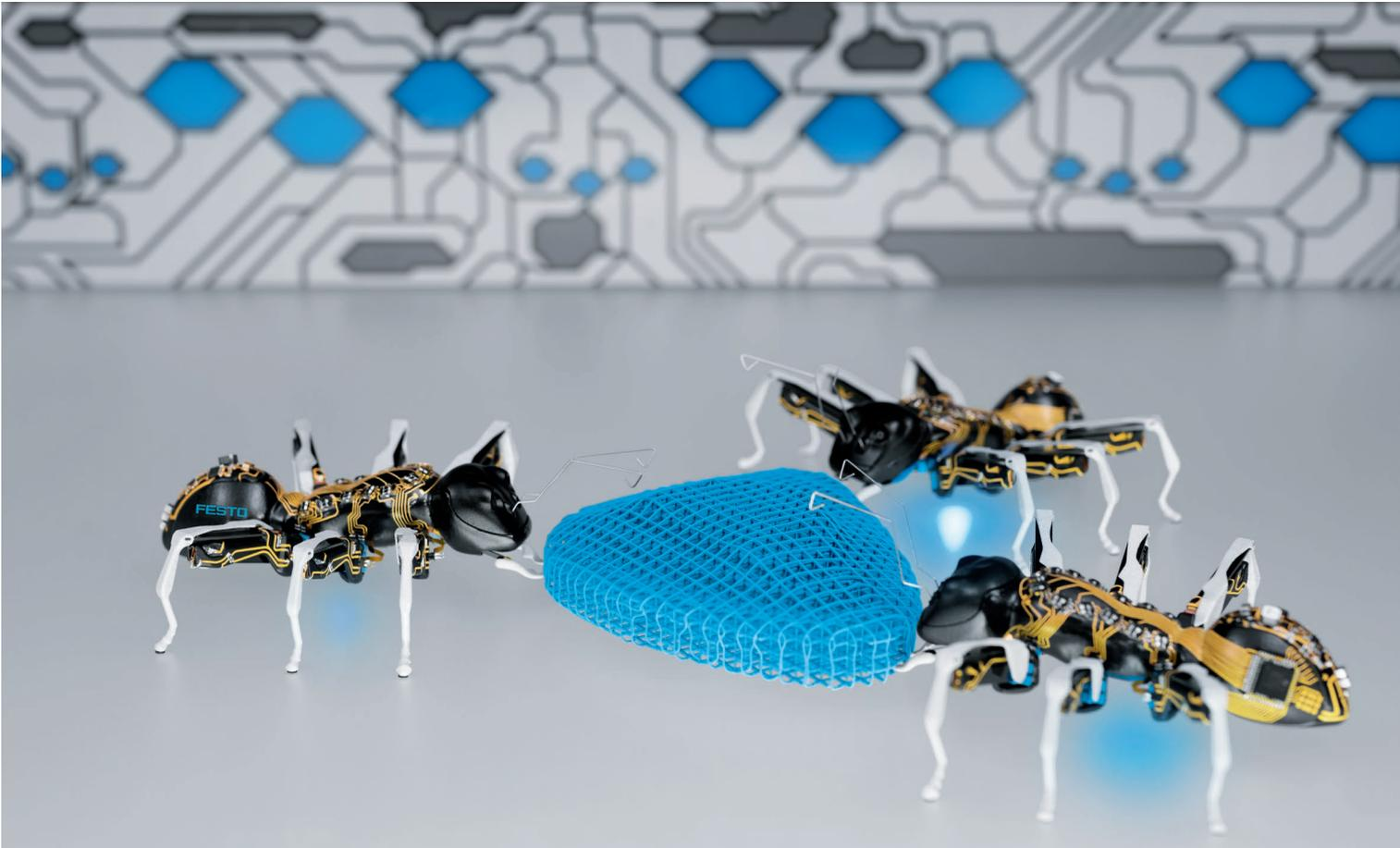
With one eye for detail and the other on the big picture: for the BionicANTs, the Festo engineers have not only taken the delicate anatomy of the natural ant as a role model. For the first time, the cooperative behaviour of the creatures has also been transferred to the world of technology using complex control algorithms.
