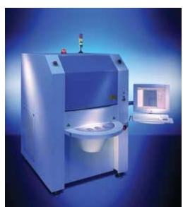
LPKF MicroLine 160: Laser system for the production of MIDs in LDS technology. Fully exploring the advantages of MIDs takes a fresh approach and some out-of-the-box thinking. That means electrical engineers and mechanical designers will be required to approach LDS MID product designs jointly.
