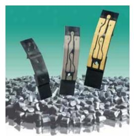
MID produced hearing aid component. Device is shown after injection molding (left), after laser activation (middle), and after metal plating (right).
