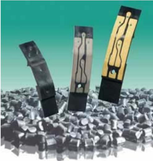
MID produced hearing aid component. Device is shown after injection molding (left), after laser activation (middle), and after metal plating (right).
