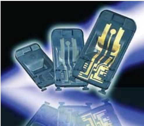
Molded interconnect device produced with laser direct structuring technology.
