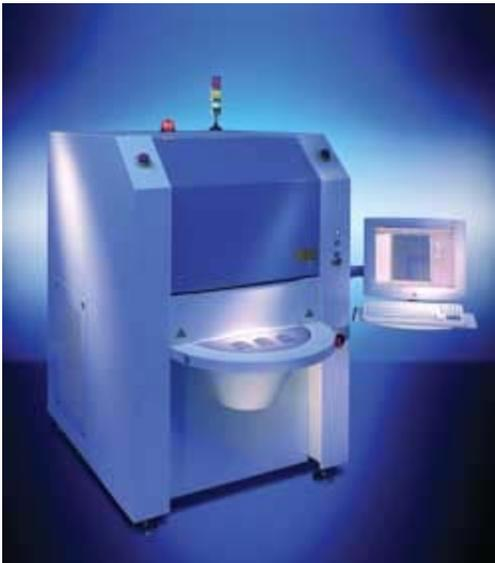
LPKF MicroLine 160: Laser system for the production of MIDs in LDS technology.
