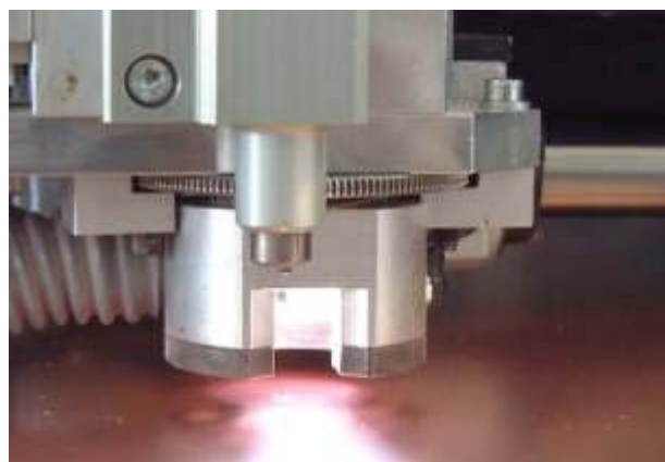
ProtoMat® circuit board plotter system with integrated head lighting
