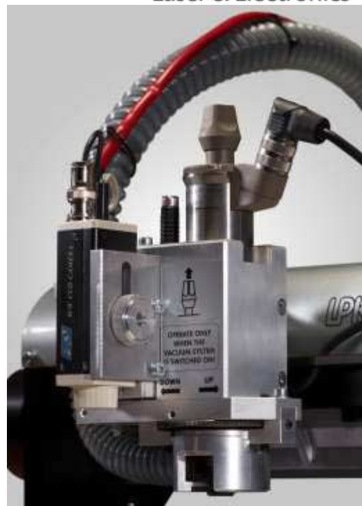
Circuit View registration camera mounted on ProtoMat® system
