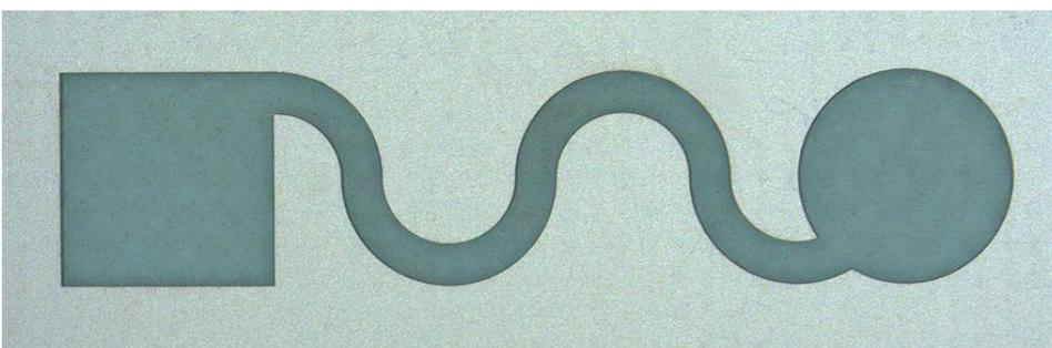
Figure 4: Top view of depth-engraved sample design in Rogers RO4003 material processed by the ProtoLaser R4
