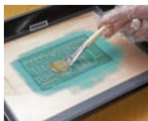
Developing the solder-resist mask
