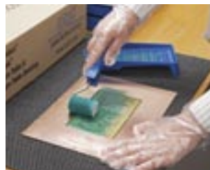
Applying the solder-resist lacquer
