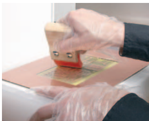
Using the squeegee to apply the paste
