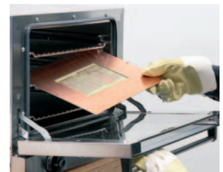
Curing the paste in a hot-air oven
