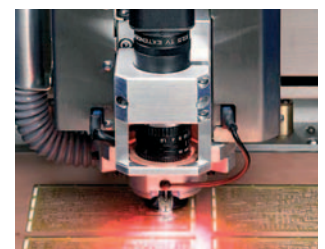
Drilling the board
