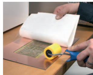
Applying the protection film
