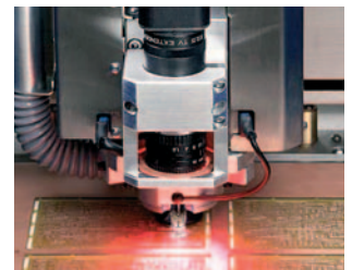
Drilling the board
