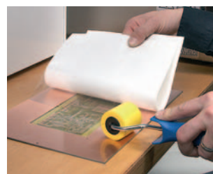
Applying the protection film
