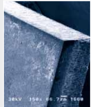
Precise cuts in sensitive materials (aluminum nitride).
