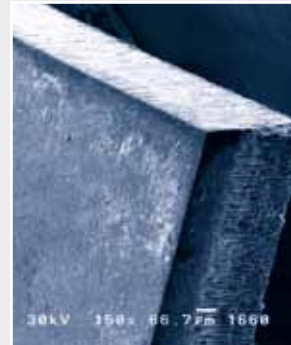
Precise cuts in sensitive materials (aluminum nitride).
