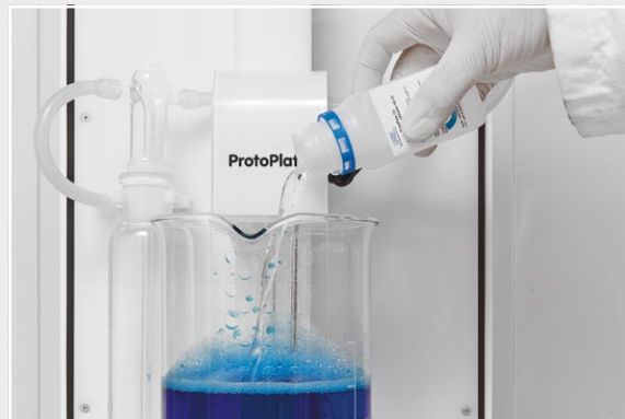
2. Pour in the activator to start the metallization bath
