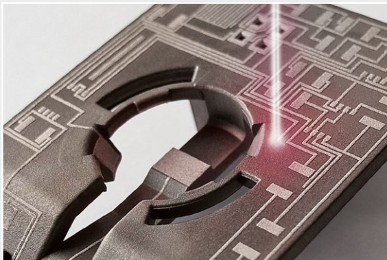
3. Structuring the circuit pattern with LPKF ProtoLaser 3D
