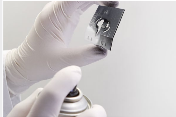
2. Painting the part with LPKF ProtoPaint LDS
