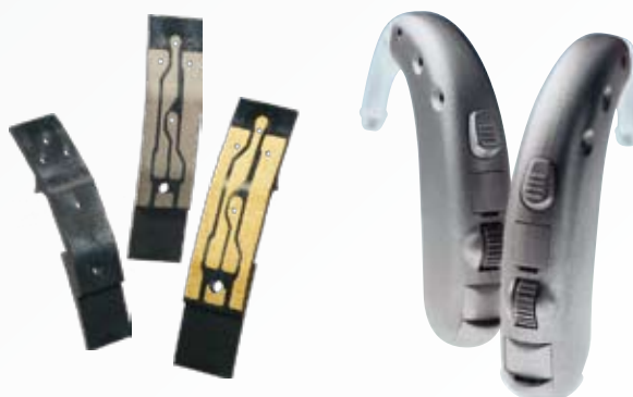
MID technology makes healthcare devices more convenient. A classical LPKF-LDS™ application: State-of-the-art hearing aids. Made by Siemens Audiologische Technik GmbH.
