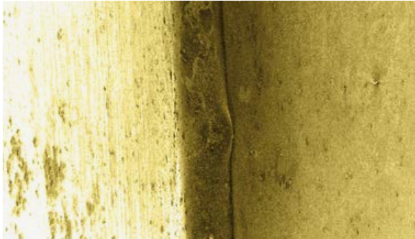
LPKF hybrid welding wins every time with a compact joint (50 x magnification).
