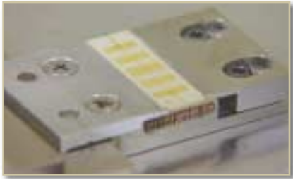
Fig. 3 The test/tune fixture of the tuning station has two positions on a precision slide for either testing or tuning.
