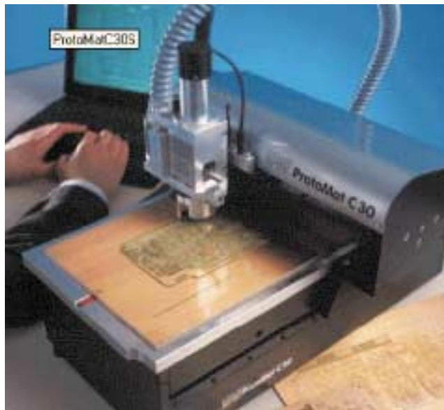
1. Compact table-top circuit-board routers can provide high precision, repeatability, and fast turnaround times on circuits fabricated on Cu-clad Teflon substrates.
