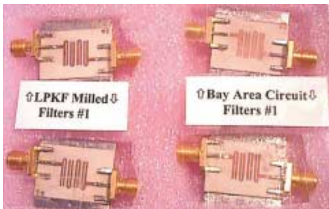
4. Using layout files from M/FILTER, mechanically milled and chemically etched filters were fabricated.
