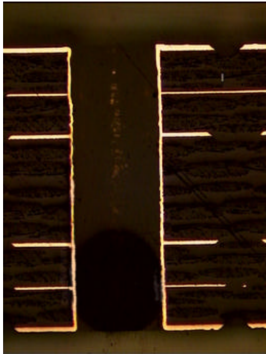
Cross section of a 6-layer board made with LPKF prototyping equipment.
