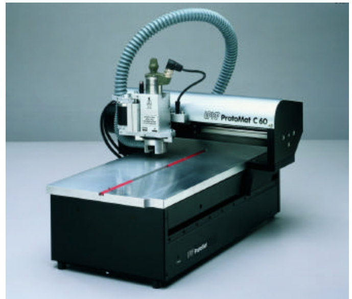
LPKF ProtoMat C60 - Circuit board plotter for in-house PCB prototyping
