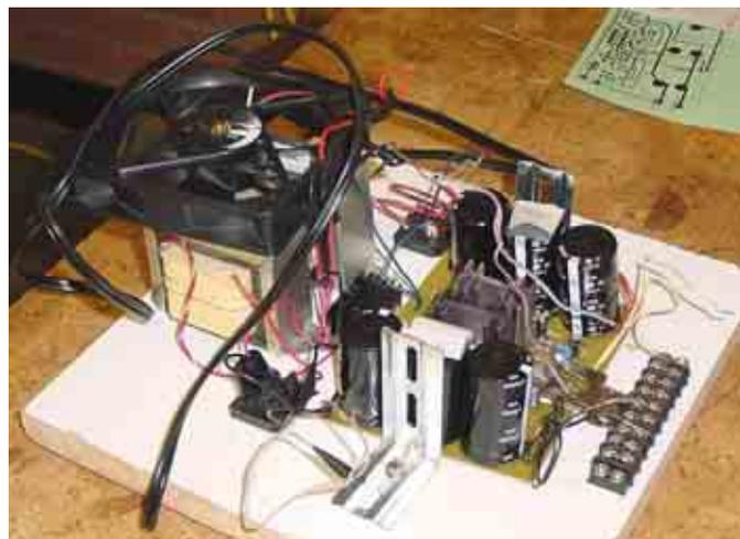
*Assembled amplifier circuit*
