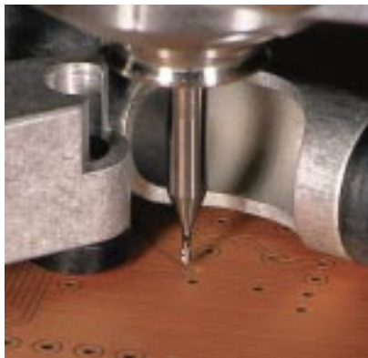
A milling bit, such as the one on this T-Tech machine, strips the copper cladding of the pc-board laminate with precision and following a software-specified path and depth.
