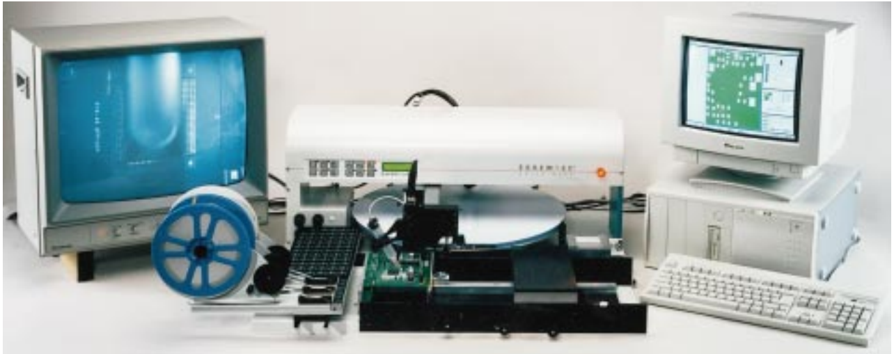
A semiautomatic pick-and-place system, such as the Expert 5000 from Manncorp, guides the operator to correct and precise component placement using a component tray as a parts source in addition to conventional tape and stick feeders.
