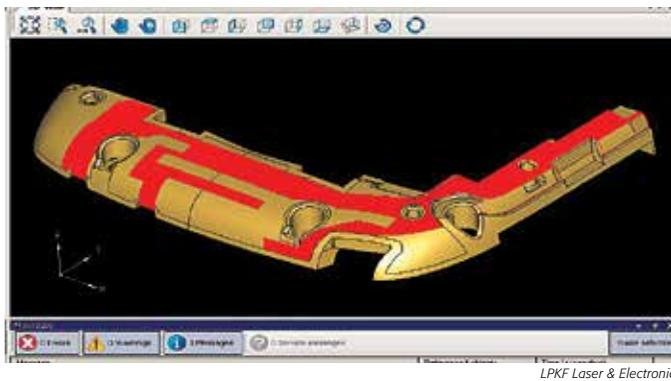
The LDS process 'writes' circuits onto parts with a laser beam striking the molded part's plastic surface.
