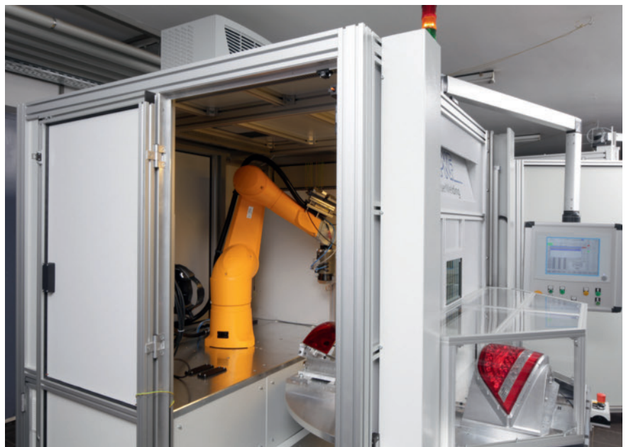
The fully automatic TwinWeld3D welding cell shortens process times, making for a flawless look and increased freedom of design in plastics welding
