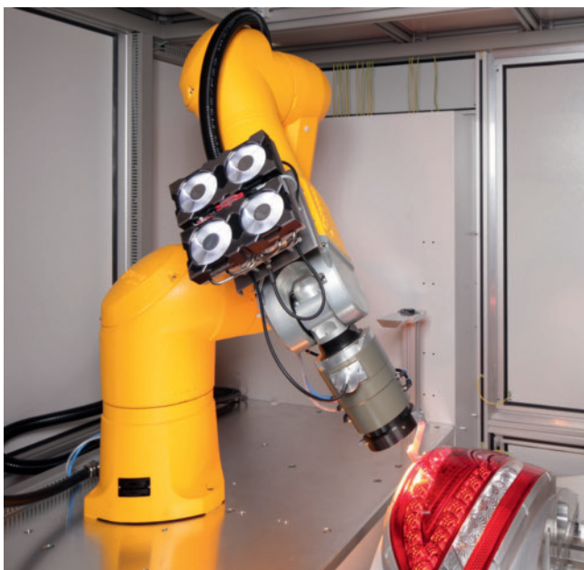
The fully automatic TwinWeld3D welding cell shortens process times, making for a flawless look and increased freedom of design in plastics welding
