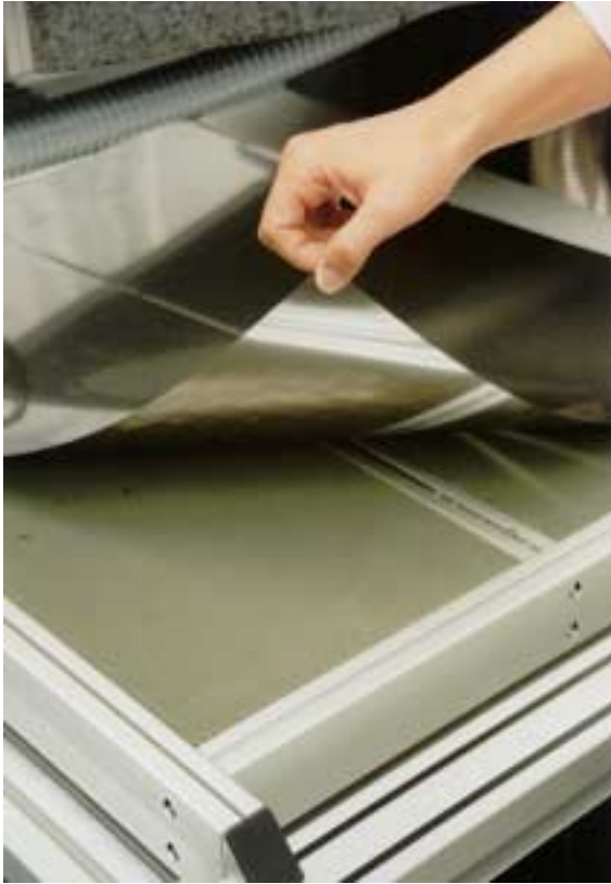
Fig 8: Easy: For the vacuum-assisted mounting of substrates, the user can choose between a honeycombed structure or perforated steel sheet
