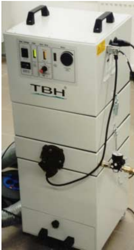
Fig 7: Labor Safety: Gases, fumes or dusts that may be generated during processing are removed and cleaned by this vacuum and filtering unit. The control system signals when it's time to change the active carbon filter
