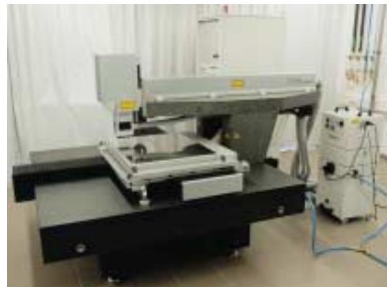
Fig 1: Solid: Precision-ground granite is widely used as a highly accurate base for high end coordinate measuring systems. The upper granite beam supports the UV-YAG laser
