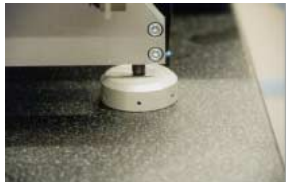
Fig 5: Precise: Frictionless air bearings on ground granite ensure high precision over the entire service life
