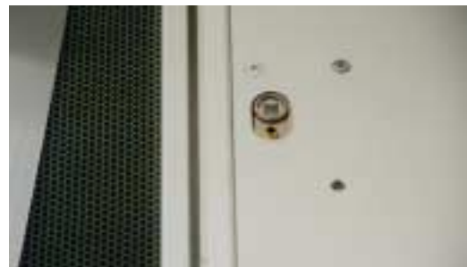
Fig 6: Time Saver: The optical positioning sensor integrated in the X-Y table provides fast and easy recalibration
