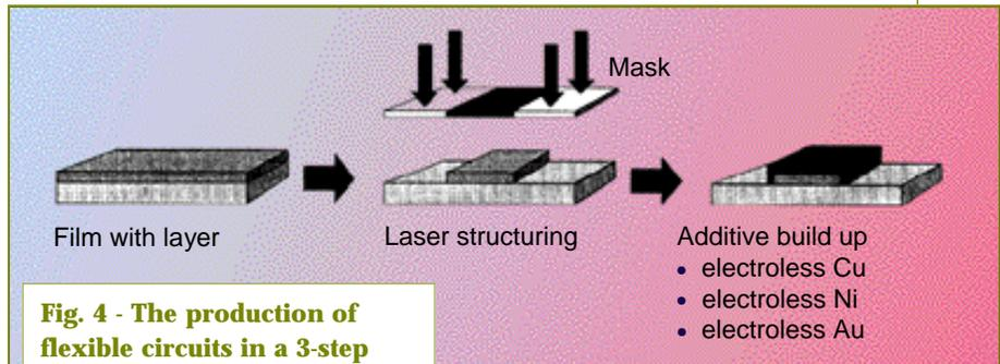
**Fig. 4 - The production of flexible circuits in a 3-step LDP process**
