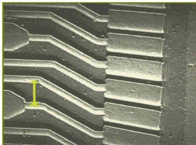
**Fig. 3 - UV-patterned Pd-doped polymer film**
