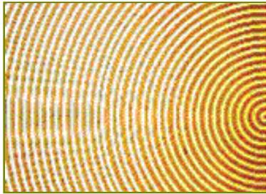
**Fig. 9 - Microcoil (15 µm lines and spaces)**
