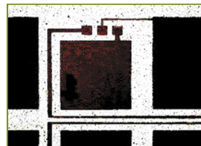
**Fig. 2 - LPD polymer film on Si-wafer. A UV laser was used to produce ≥30 μm features**
