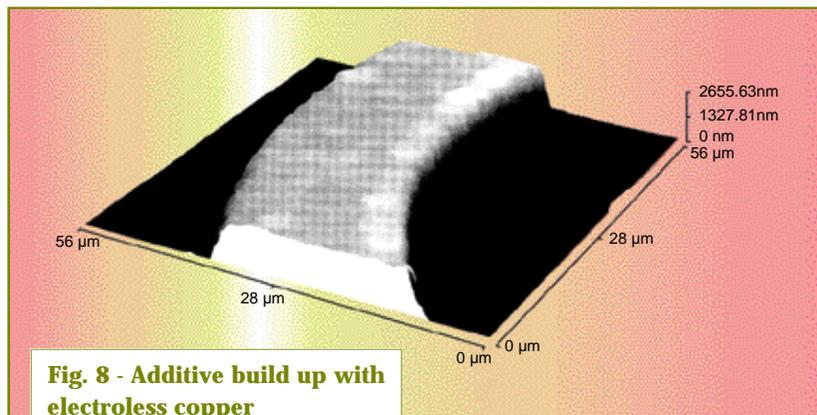
**Fig. 8 - Additive build up with electroless copper (19 µm line width)**
