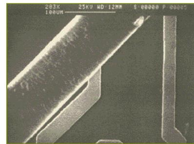
**Fig. 7 -  $15\mu\text{m}$  (0.6 mil) ablated tracks compared with human hair**
