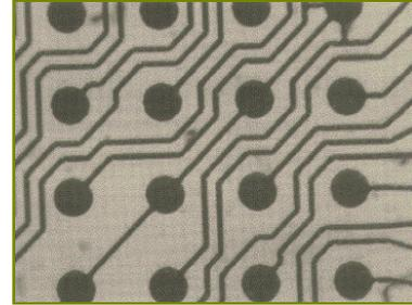
Fig. 12 shows an LDP interposer. This was completed as a CSP demonstrator and has been tested successfully according to the general reliability test for electronic components.
