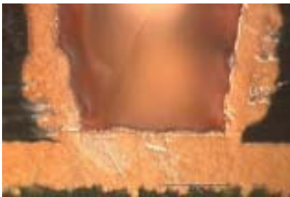
Fig. 3: Flawless connection throughout the entire bottom of the via. (Photo: Fachhochschule Stralsund - University of Applied Sciences)
