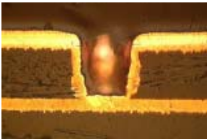
Fig. 2: Microvia in FR4 with 1 layer of 1080 glass reinforcement. (Photo: Fachhochschule Stralsund - University of Applied Sciences)
