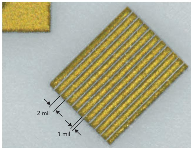
**FIGURE 2.** UV laser creates circuit traces so small a microscope is needed to view them.
