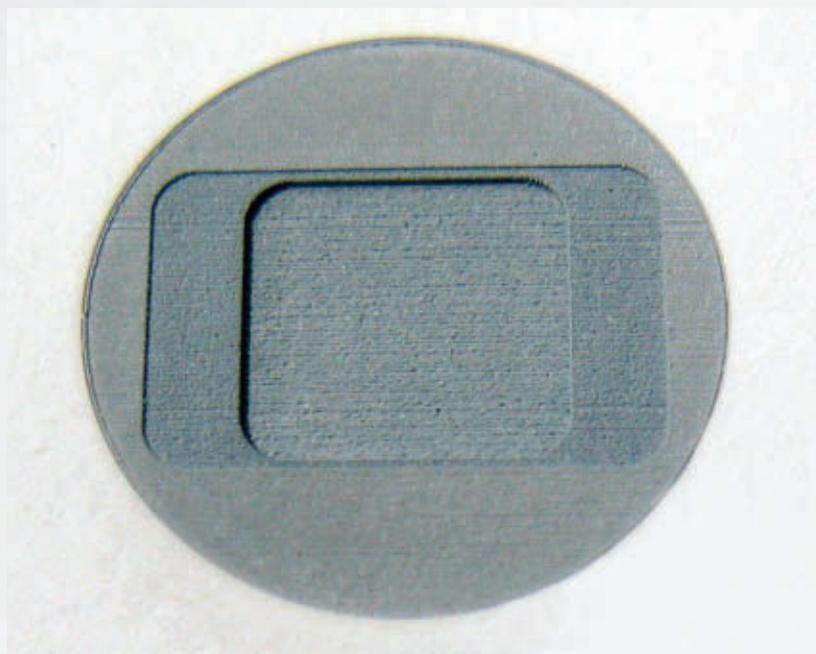
**FIGURE 6.** In this polyethylene material, the laser was set to create one step at a depth of 2 mils, another 8 mils below that, and another 10 mils below that.
