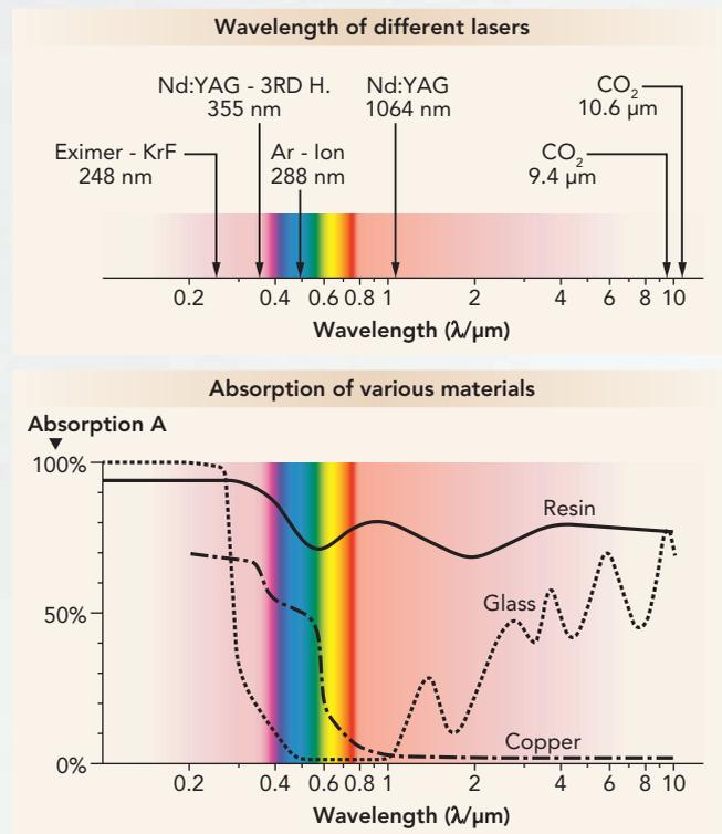
**FIGURE 1.** Absorption rates of three common PCB materials for six types of lasers.
