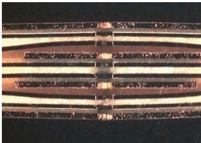
**FIGURE 4.** In this cross section, a 4 mil hole has been drilled in a 14 mil multilayer board.
