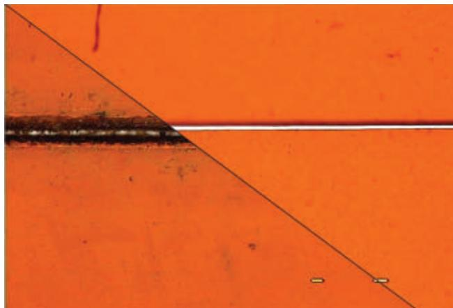
**FIGURE 3.** A flexible substrate (polyimide) cut with a (left)  $\text{CO}_2$  laser and (right) UV laser.
