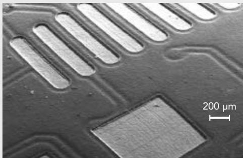
**FIGURE 5.** A skiving application performed by a UV laser.
