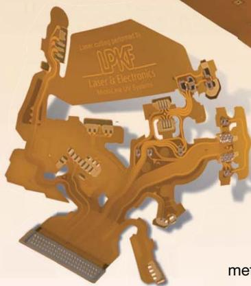
**FIGURE 1.** Flexible printed circuit cut with a UV laser system.
